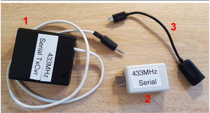
This image shows the Radio Serial Sender Unit connected to the 3.5mm console socket of a project and a mobile phone using the Radio Serial USB Unit through an OTG USB Bus master cable shows the console (with logging information) of the project.
