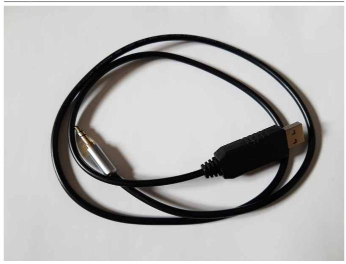
Below, I have used the American notation of Tip, Ring and Ground (which ties in nicely Tx, Rx, Gnd) and to clarify I have also equated these with MISO/MOSI notation to clarify the direction of each without ambiguity. This setup has no problem with 38.4KBaud, I have not tried it higher as I have never needed it but I can't imagine too many problems.
