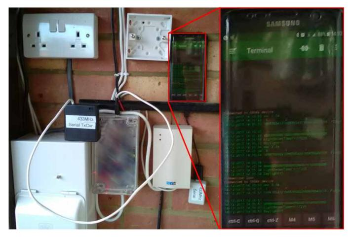
The USB Terminal App for android used above recognizes the common and ubiquitous CH340G, FT231/2, CP210x and PL2303 devices natively. You might have to hunt around for a compatible Apple
