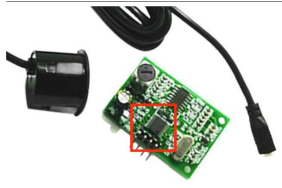
Confusingly the silk screen marks the pins on both types as Rx/Tx and Trig/Echo so no help there :o(
