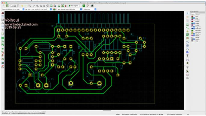
J1 is the connector that plugs into the micromite backpack.
