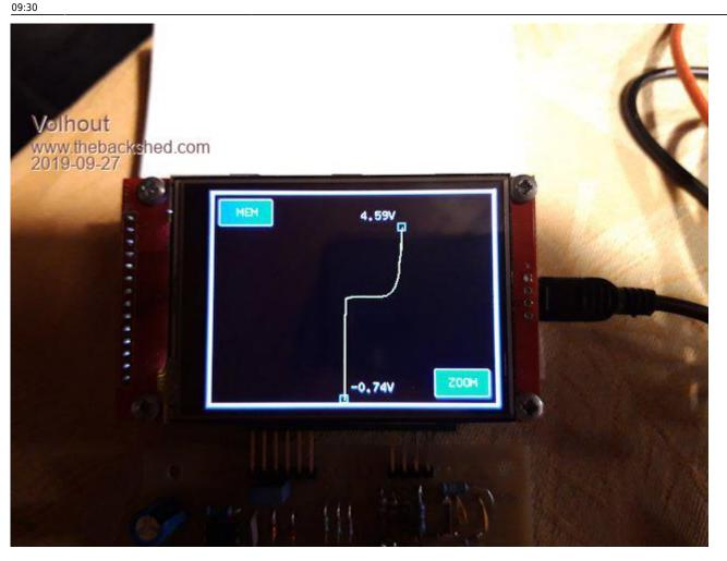
There are 2 buttons: MEM: this button stores the current waveform, and displays it in red, as a reference. This would be the waveform of the "known good" circuit. ZOOM: this button zooms in at the center, to allow more detail if low voltage circuits are probed.
